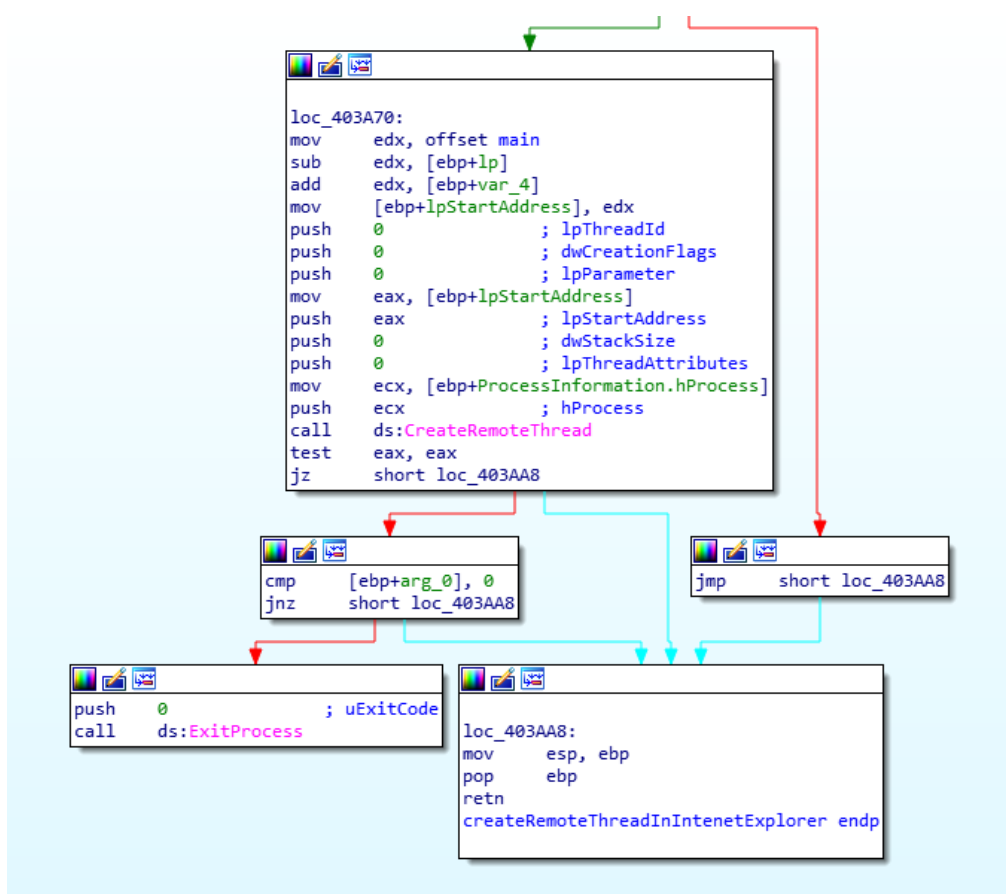
Figure 19: an InternetExplorer process was created by the malware and memory has been allocated. This figure shows the creation of the remote thread which finalizes the process injection. More information regarding this process injection technique can be found here .
